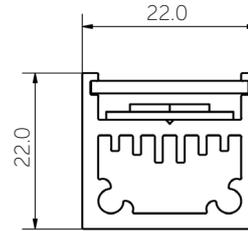
Sonny Side Up 22 is a purpose-designed powerful uplight profile. Don't be fooled by its petite size as it packs a mighty punch of light up to an amazing 2460 lumens per metre. Both wire and rod suspensions are available for the Sonny Side Up 22 extrusion.
