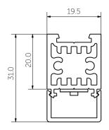
The Sideways Sally 20R extrusion is a compact uplight/downlight solution providing powerful LED lighting. A versatile system suitable for various mounting options, Sideways Sally 20R can be surface mounted, wall mounted and suspended. The concealed mounting clip provides a quick and secure fixing to joinery. Both wire and rod suspension options are available for the Sideways Sally 20R extrusion.
