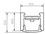
The Downhill Dan 14 extrusion is a compact solution providing dot-free lighting. A versatile system suitable for various mounting options, Downhill Dan 14 can be surface mounted, recessed and suspended. Both wire and rod suspension options are available for the Downhill Dan 14 extrusion and the recessing system for plasterboard ceilings and walls, creates a perfect trimless recessed finish every time.
