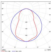
C00 . C27 Polar curve for 1890 lumen LED strip with opal diffuser.
