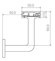
Richie Rail 17 is a unique illuminated handrail system. CNC machined wall brackets provide a beautiful finish and make for quick installation. Hollow wall brackets conceal the power supply to the LED strip, and the low voltage input makes the handrail safe to touch. Richie Rail 17 is suitable for use on residential and commercial stairs and thoroughfares.
